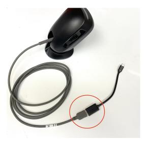
d. If needed, remove 1 of the 2 port covers located on the left and right backside of your tablet to expose the micro USB ports. Insert the micro USB cable into the left or right micro USB port. Once the scanner is plugged in, you will hear 3 ascending beeps and red light will appear on the top of the scanner.
