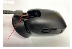
c. Insert the male USB end of the cable into the female USB end of the adapter.
