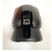
b. Insert the ethernet end of the cable into the port on the lower back of the scanner. Be sure that locking tab on the cable is facing down
